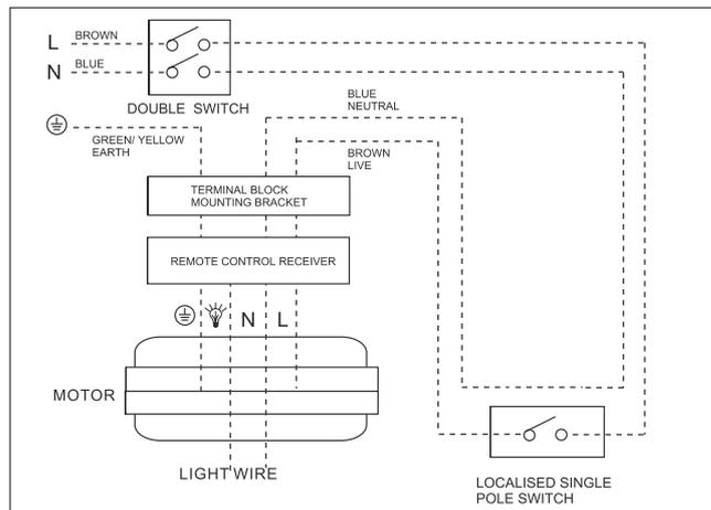
All pole disconnection switch must be included in the fixed wiring.
