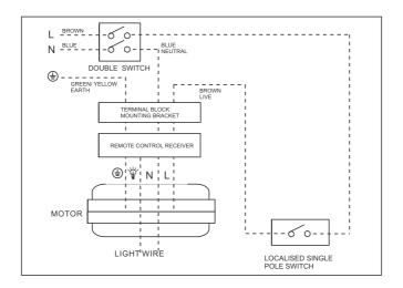
Step 1: Connect the EARTH wire to the terminal port marked "
